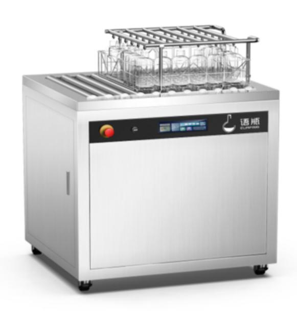
Application: automatic filling system for canning of drinking bottles in animal laboratories.
