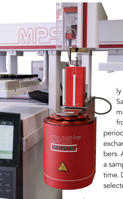
DHS large sample containers with pressure valves are available in the sizes: 250 mL, 500 mL, and 1 L
