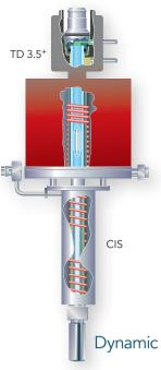
The TD 3.5<sup>+</sup> is coupled directly to the Cooled Injection System (CIS): The "Liner-in-Liner" design ensures best possible analyte transfer to the GC column without discrimination or cross contamination. The builtin TD 3.5<sup>+</sup> alignment support simplifies liner replacement and mounting.
