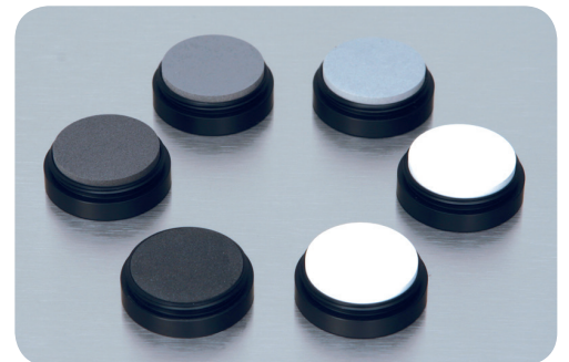
Set of Labsphere reference standards for photometric linearity test (according to USP <1119> and Ph. Eur. 2.2.40).
