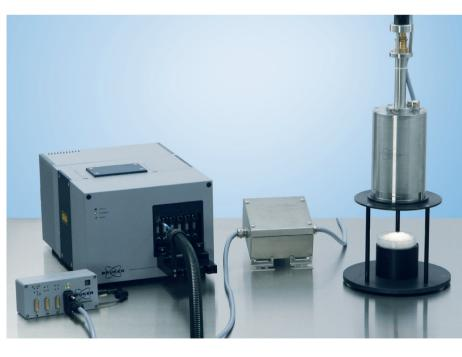
Ex-proof sensor head connected to a standard MATRIX-F spectrometer
