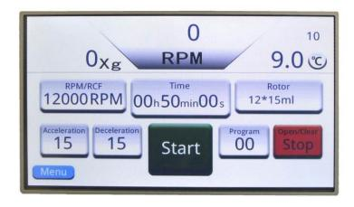
The glove friendly touchscreen display gives you ease of control and a modern feel. An advanced microprocessor controls allow for setting/displaying of the rotational speed in either RPM or RCF. It is splash-proof and protects the inner electronics from external elements.
