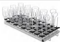
PLYT-50 50-Position Spray Bottle Module Bottle volume: 10 - 100ml Clean erlenmeyer flask, volumetric flask, triangular flask, flask, etc. With three-petal flower basket bottle holder and cross bottle holder. Each module can clean 50 volumetric flasks of 50ml
