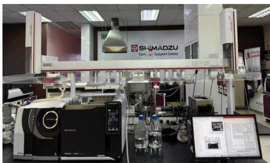
Figure 1: Full setup of Shimadzu GCMS-QP2020 NX with Gerstel MPS Workstation
